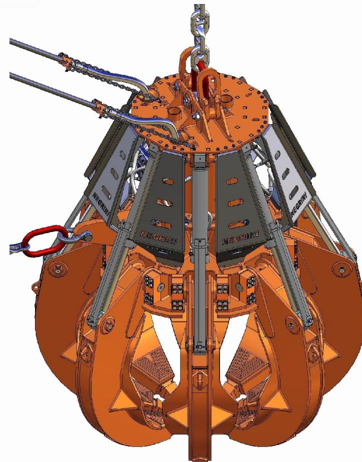
Changing the shells varies the characteristics of the grab. It is possible to fit standard shells with welded Hardox teeth protected with surface hardening, shells with replaceable teeth, completely closed shells, or with profiles as requested.
