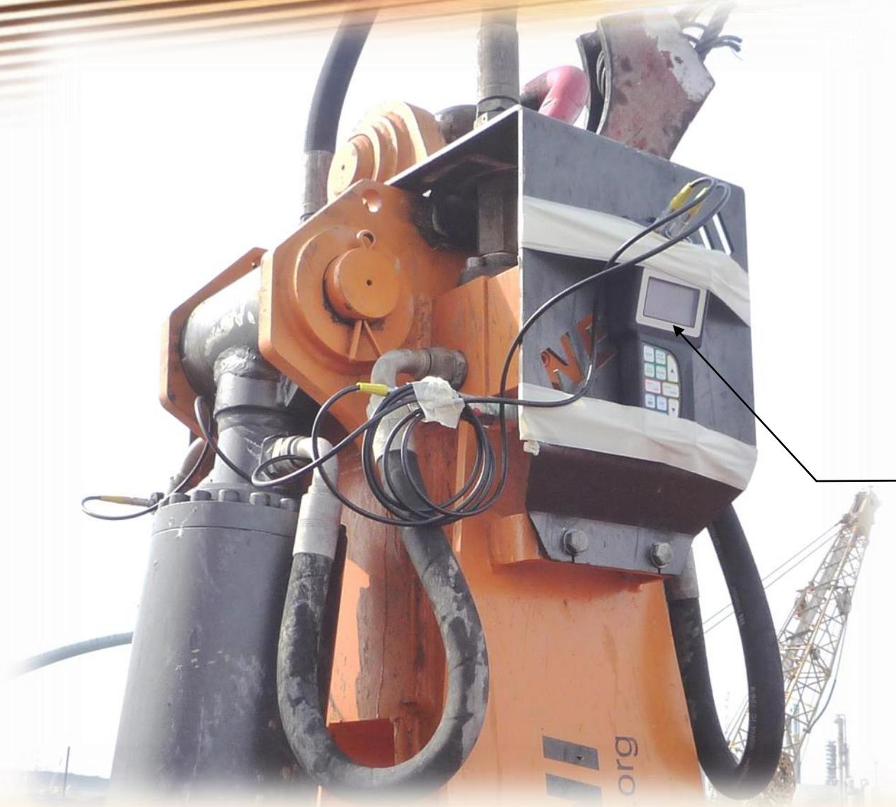
When possible we carry out operating tests using electronic instruments fitted to the bucket in order to check the evolution of flow rates, pressures, back pressures, and good general operation.
