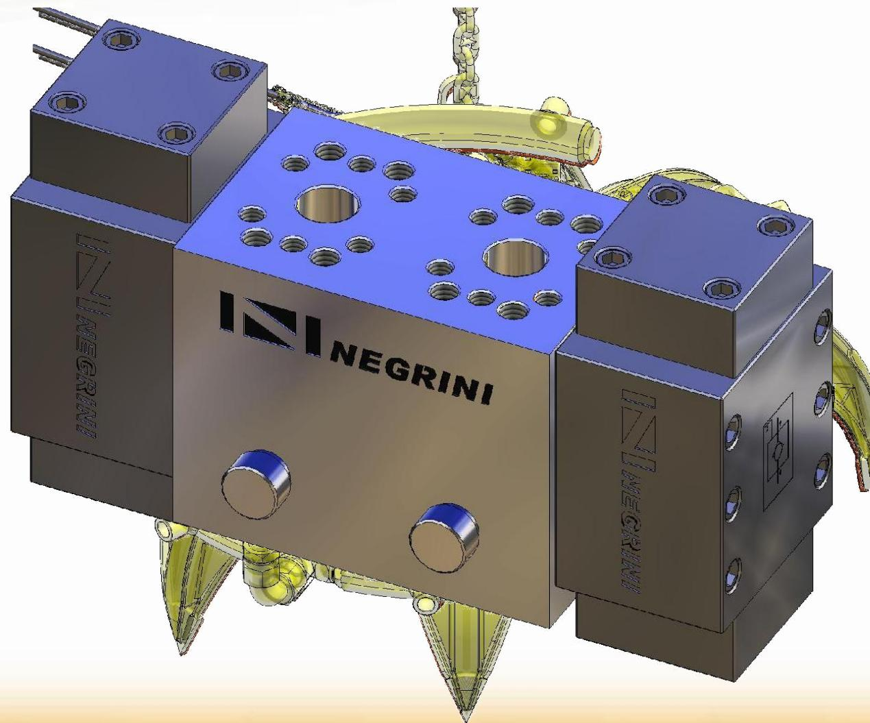
The high shell opening speed is provided by a special hydraulic system solidly fitted inside the bucket. This also holds the large valves that ensure the hydraulic locking of the system. The hydraulic system limits back pressure to 7 bar, eliminating harmful energy wastage and hydraulic hammer effects, allowing the pipes and winders to remain in an idle state. The bucket can be used in transverse or longitudinal orientation.
