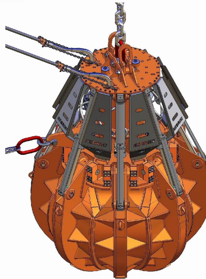
Changing the shells varies the characteristics of the grab. It is possible to fit standard shells with welded Hardox teeth protected with surface hardening, shells with replaceable teeth, completely closed shells, or with profiles as requested.
