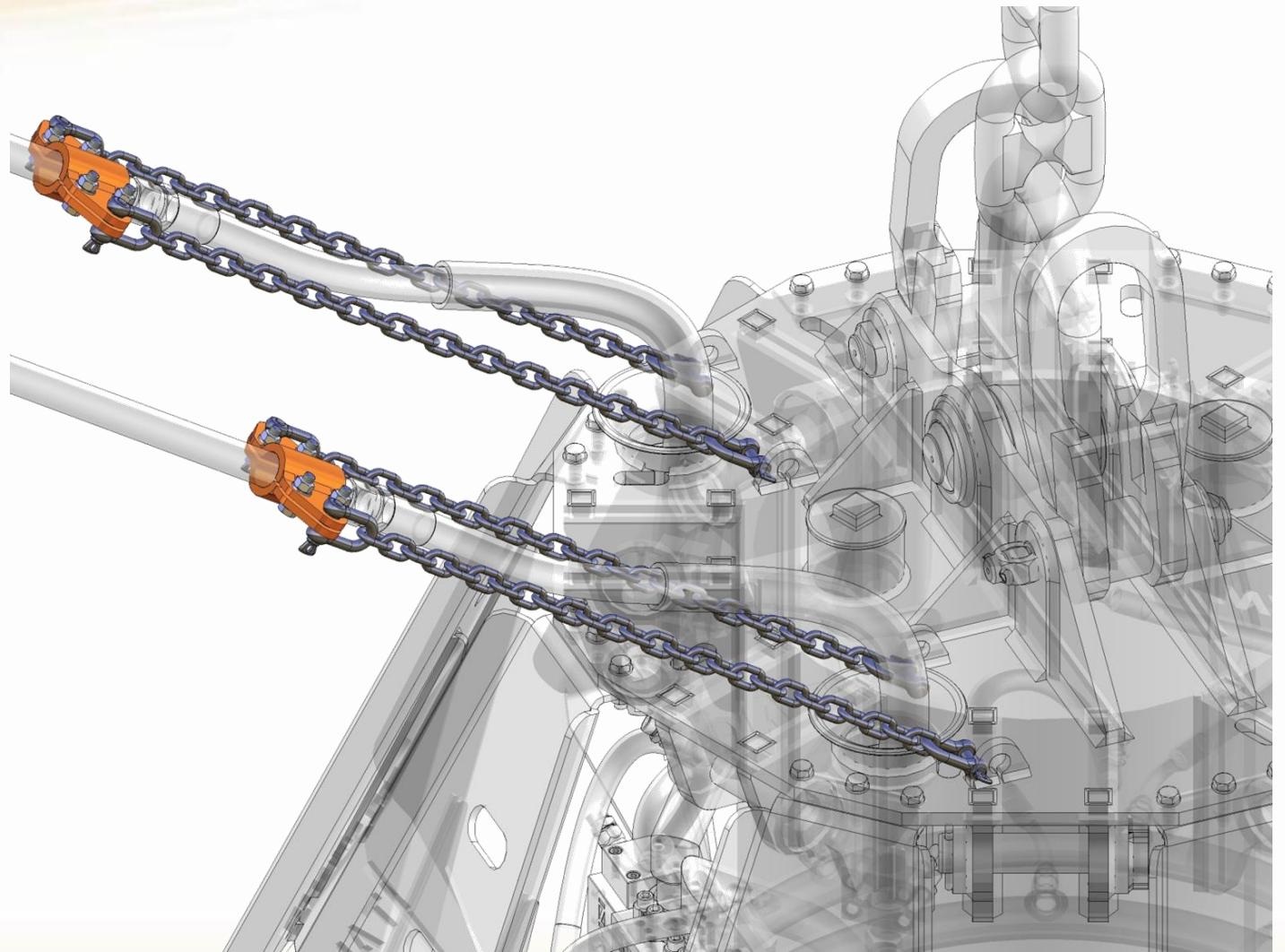
The hydraulic supply pipes must not be put into traction and to avoid this we use chains and clamps that restrain the pipes from the machine.
